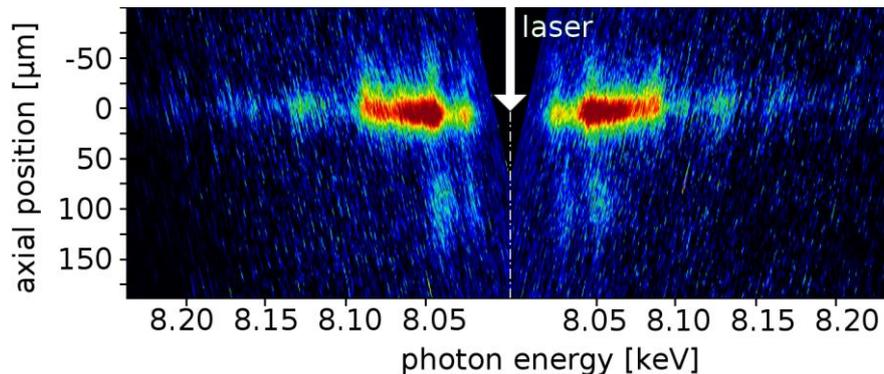
Spatially resolved Cu  $K\alpha$  spectrum recorded by a vertical-geometry Johann spectrometer.
