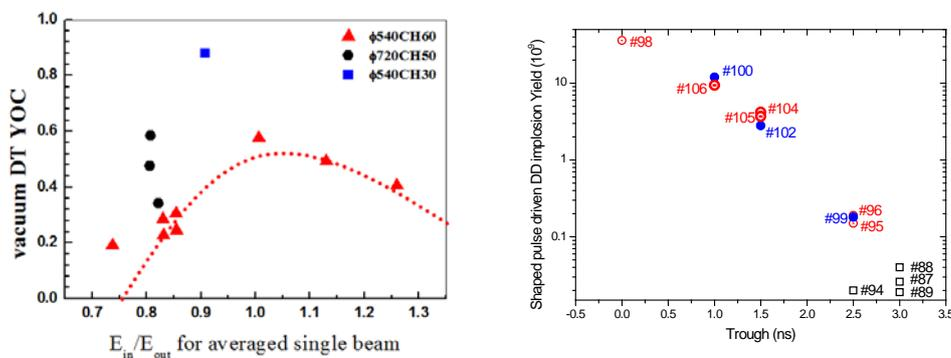
Figure 1: YOC vs. inner/outer cone fraction of laser energy for implosions driven by square pulse(left) and the neutron yield vs trough length for implosions by shaped pulses (right). Here different symbols stand for different size of hohlraums.
