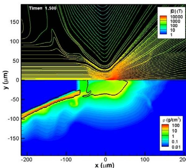
Figure 1: Magnetic-field lines and strength in tesla (upper panel). Mass-density contours ( $\text{g}/\text{cm}^3$ ) at 400 ps before maximum compression. Solid black lines indicate material contact surface between CD, DT, and Au (lower panel)
