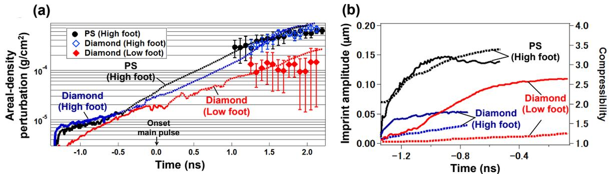
Figure 1: (a) Areal-density perturbation growth for targets from experiments (symbols), and from the PINOCO-2D simulation for each experimental configuration prior to the foil acceleration (solid curves) and after the acceleration (dotted curve). (b) Temporal evolution of imprint spatial amplitude (solid curves) and target compressibility (dotted curve) with 2D simulation (PINOCO).
