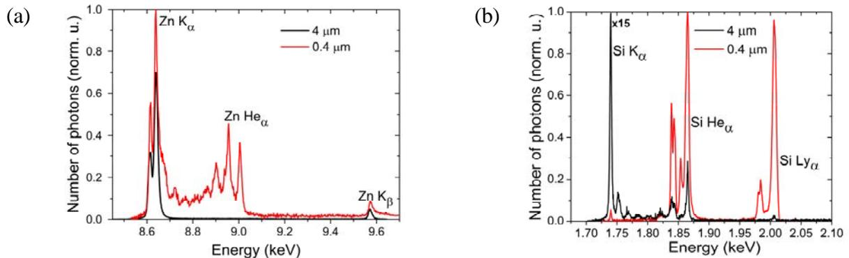
Figure 1: K-shell emission spectra from ZnO NW (a) and Si NW (b) targets generated by ultrashort relativistic laser pulses with long (red) and short (black) wavelengths.
