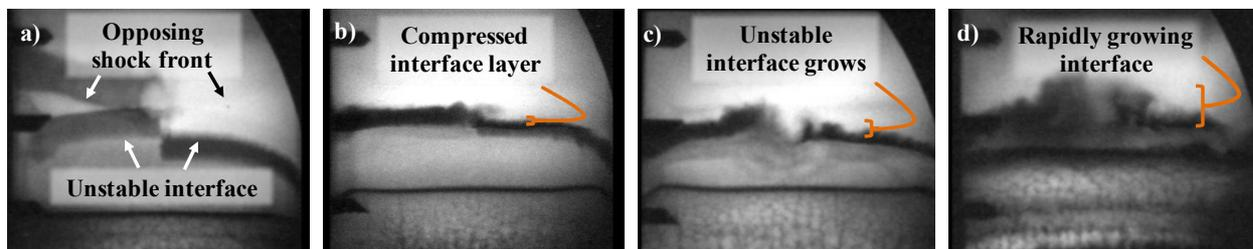
Figure 1: Four images capture the pre- and post-reshock interface growth. In each figure, the initial shock is launched from the bottom of the image, traveling upward, and the opposing (“reshock”) is traveling from top to bottom. a) The unstable interface is measured 2 ns prior to reshock, establishing the initial mix width. b) – d) In images captured at 4, 10, and 18 ns after the reshock, the unstable interface is seen to be compressed, followed by a period of rapid growth.
