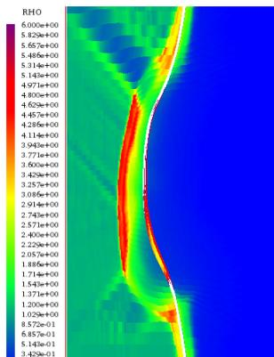
Figure 1 : Density map from a CHIC simulation of a CH target irradiated by three LMJ quads (t=6.2 ns)
