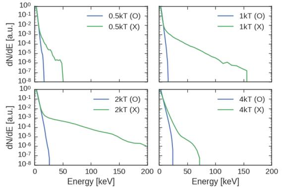
Figure 1: Electron energy spectra in O- and X-wave propagation under various magnetic field strength
