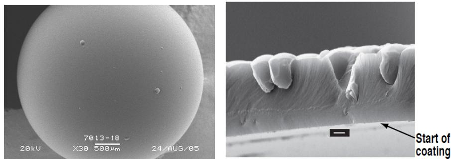
Figure 1: Internal Capsule Defects. Right picture is taken from Ref. [1]
