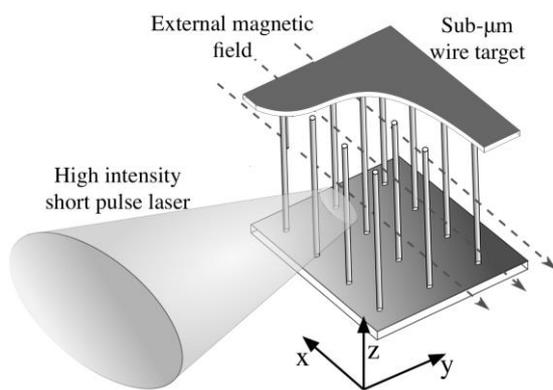
Fig.1 Magnetic confinement system by utilizing the structured material.
