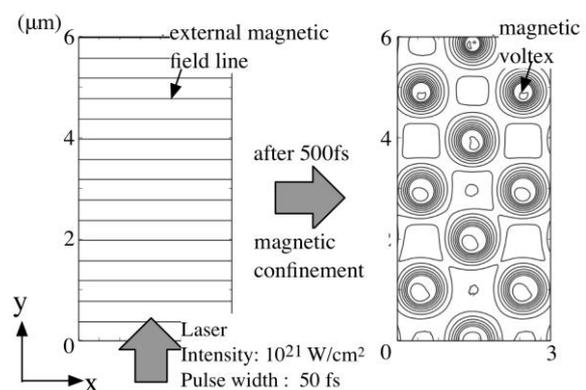
Fig.2 Generation of magnetic vortex around the rod in 2D PIC simulation result.
