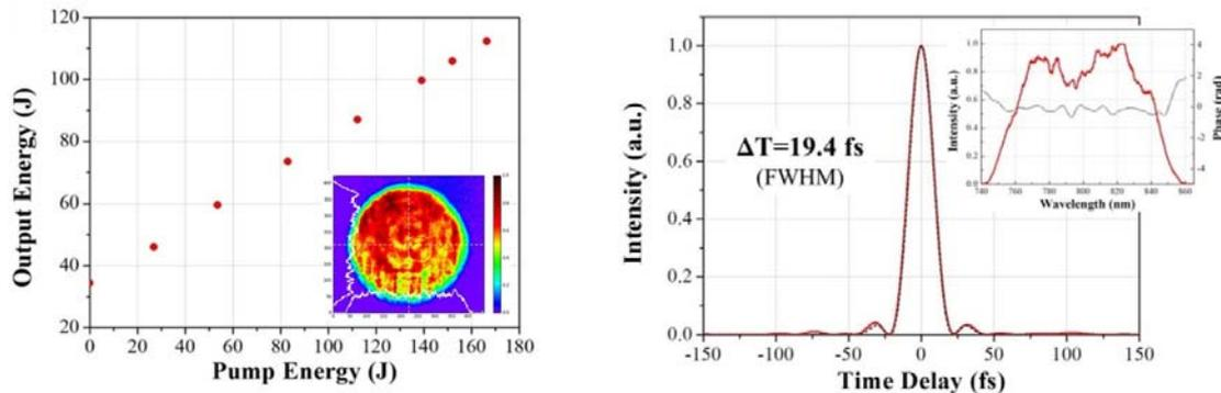
Figure 1: Measured output energy as a function of pump energy in the final booster amplifier (left) and reconstructed temporal profile of the 4 PW laser (right).
