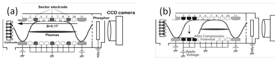
Figure 1: Schematic configuration of a Malmberg-Penning trap. Electrons are compressed longitudinally to the half of an initial length by manipulation of the confinement electric potential.
