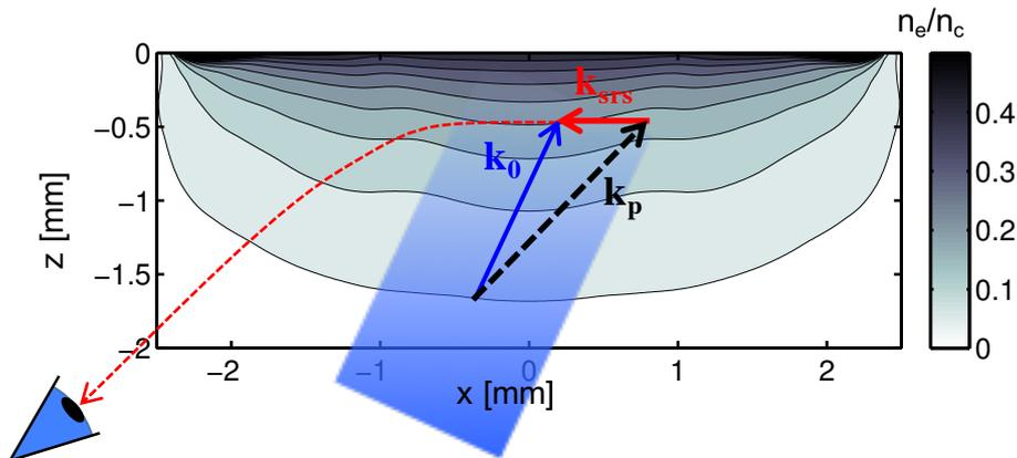
Figure 1: Raman side-scatter geometry for a planar target experiment (density contours in grey color-scale, from DRACO simulations), with a laser beam incident with wave-vector  $\mathbf{k}_0$  (in blue) driving a plasma wave ( $\mathbf{k}_p$ ) and a Raman scattered wave  $\mathbf{k}_{srs}$  perpendicular to the density gradient.
