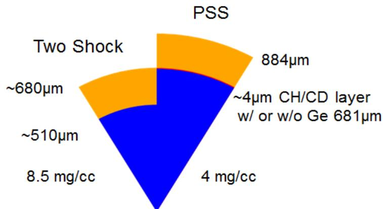
Figure 1: Comparison of the two-shock and PSS capsule designs.
