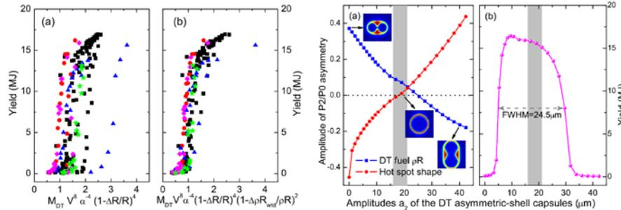
Figure 1: Left figure shows a new metric of the low mode asymmetry, and the right figure show the DT asymmetric-shell capsule design can significantly improve the implosion performance.
