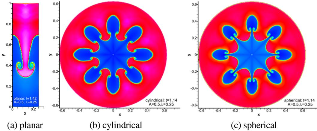
Figure 1: Two-dimensional numerical results of the compressible Rayleigh-Taylor instabilities with the same Atwood number  $A = 0.5$  and wavelength  $\lambda = 0.25$  in planar, cylindrical, and spherical (rotationally symmetrical) geometries.
