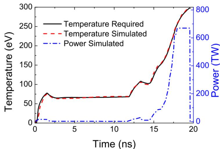
Fig. 1 Radiation temperature (dashed: required by the CH Rev5 capsule, solid: from 2D simulation) and laser power (dash-dotted) for the designed octahedral spherical hohlraum with  $R_H = 5 R_C$  and  $R_L = 1.2$  mm.
